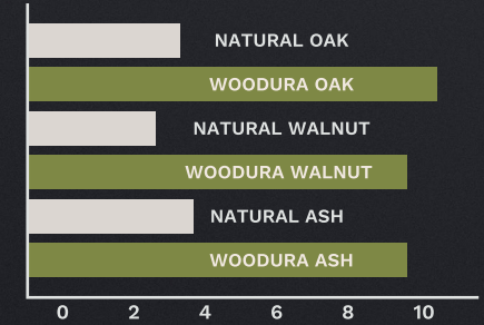
Results from the Brinell Hardness Test
